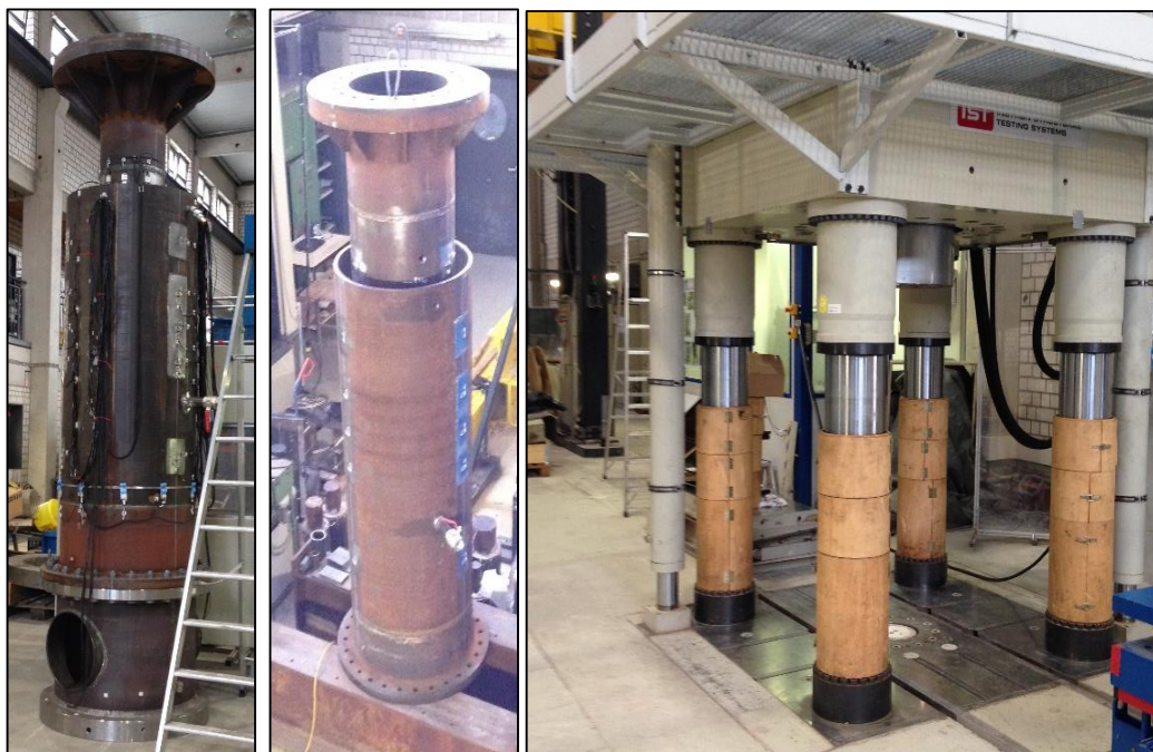
Figure 8: Large scale jacket, tripod specimen and test rig (from left to right)
