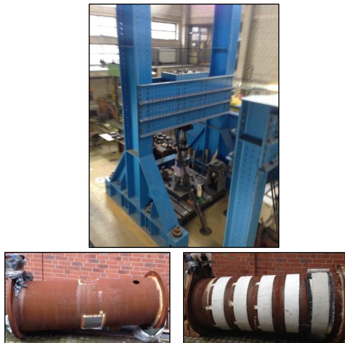
Figure 6: Parts from large scale bending specimen ( monopiles )
