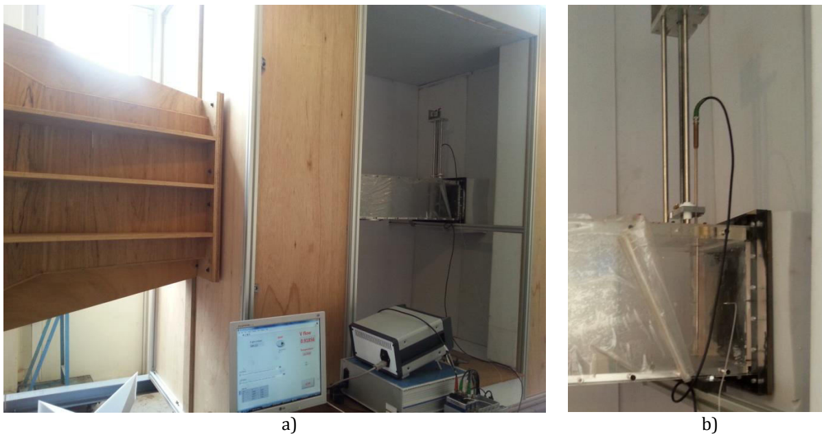
Figure 1. Wind tunnel facility: a) view of the test section enclosed inside an acoustically isolated chamber; b) view of the hot wire probe installed inside the test section and wall pressure tap.
